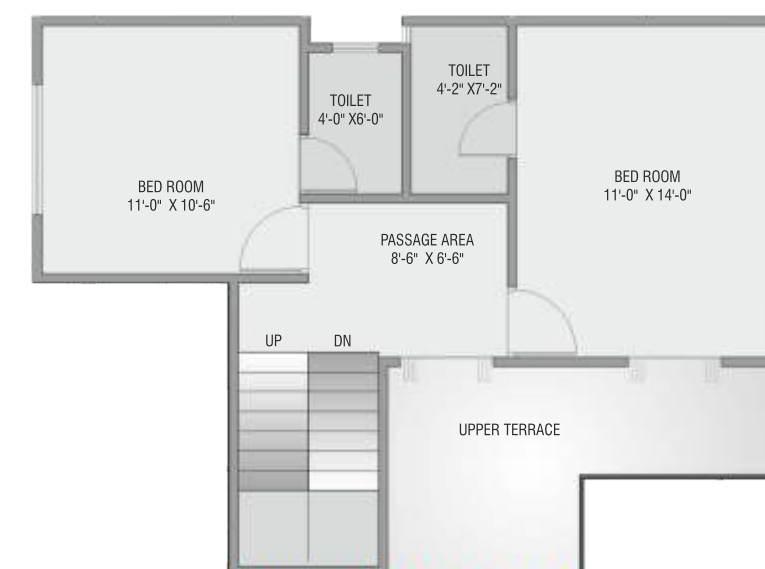
Penthouse (upper level) (Tower : C)
