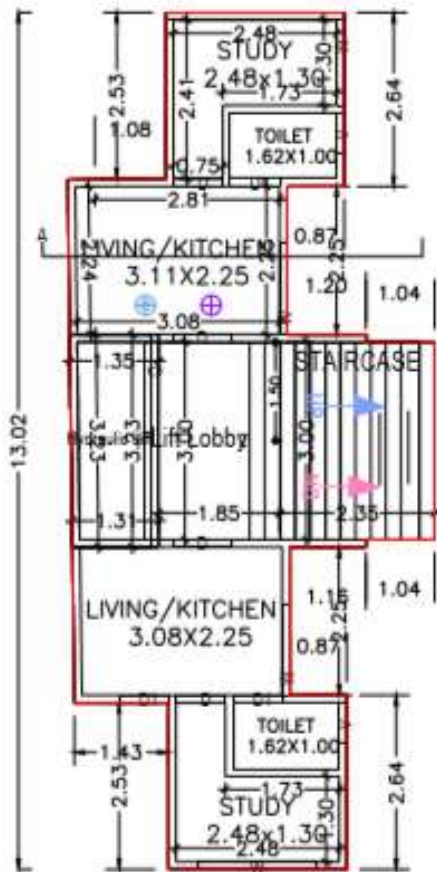
TYPICAL - 2, 3, 4, 5 FLOOR PLAN (Proposed) (SCALE 1:100)
