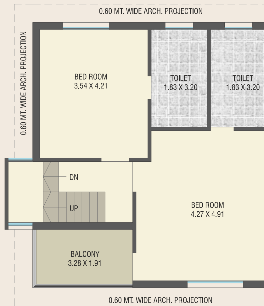
FIRST FLOOR PLAN [ TYPE - B2 ] BUILT UP / F.S.I. AREA : 69.66 SQ.MT. CARPET AREA : 57.39 SQ.MT.
