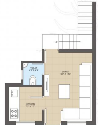
C- TYPE(Tenement) Ground Floor Plan (Unit No - 10, 13) Minimum Plot Area = 596 SQ.FT. Super Built Up Area = 315 SQ.FT
