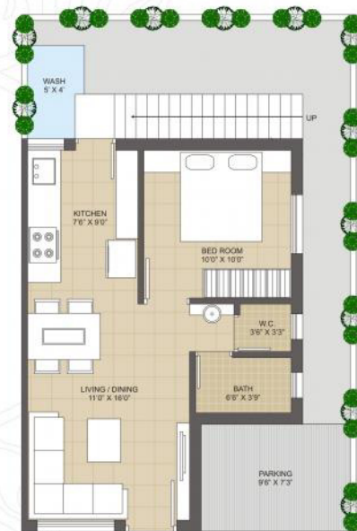
B- TYPE (Tenement) Ground Floor Plan (Unit No - 11, 12, 14 to 21) Minimum Plot Area = 740.00 SQ.FT. Super Built Up Area = 561.00 SQ.FT
